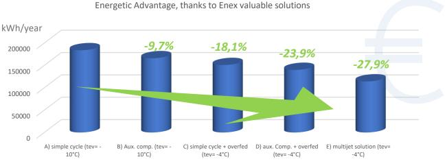
■ Energy consumed in kWh/year for a commercial refrigeration plant of 100 kW MT/30 kW LT, Located in Bari – Italy
